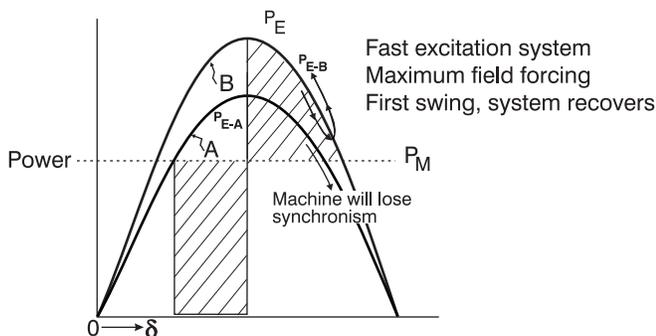
Fig. 8. Effect of High Initial Response Excitation System
