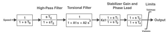
Fig. 14. Speed-based Stabilizer
