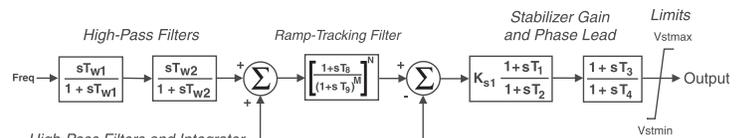
Fig.16. Block Diagram of Dual-Input Power System Stabilizer
