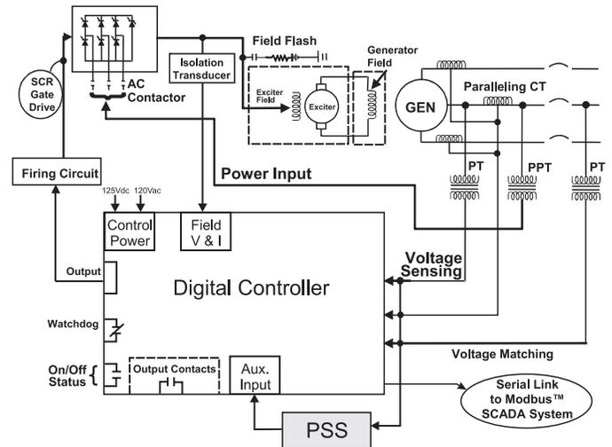
Fig. 13. Block Diagram of Excitation System and PSS
