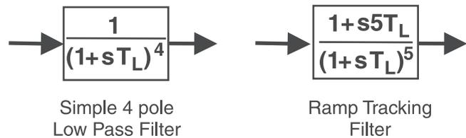
Fig. 20. Filter Configurations for Derived Mechanical Power Signal
