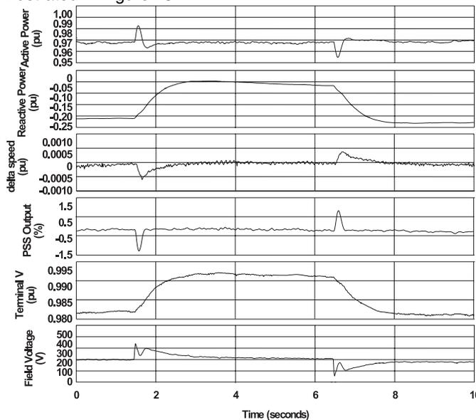
Fig. 25. On-line Step Response, Basler PSS-100  $K_s=7.5$ , 92MW Hydro Turbine Generator
