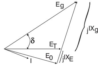
Fig. 4. Phasor Diagram, Generator tied to infinite bus
