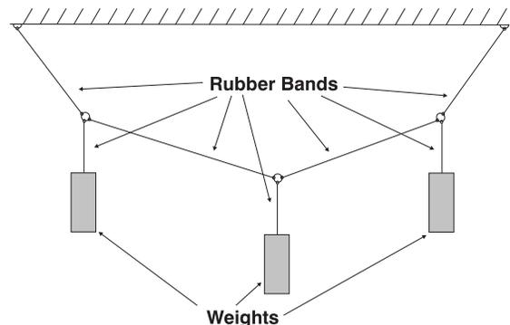
Fig. 5. Rubber Band Analogy
