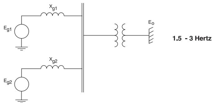
Fig. 9. Inter-unit Oscillations
