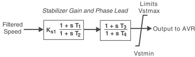
Fig. 21. Output stage of PSS to AVR
