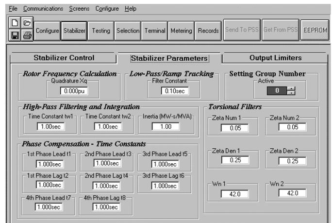
Fig. 26. Setup Screen for Power System Stabilizer Tuning
