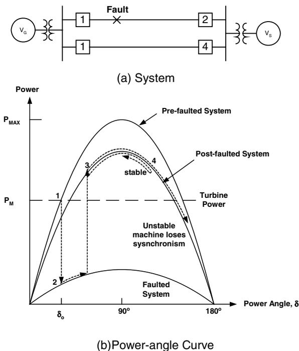
Fig. 6. Transient Stability Illustration
