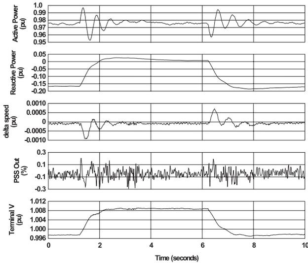
Fig. 15. On-line Step Response, Frequency Type PSS  $K_s=6$ , 92MW Hydro Turbine Generator
