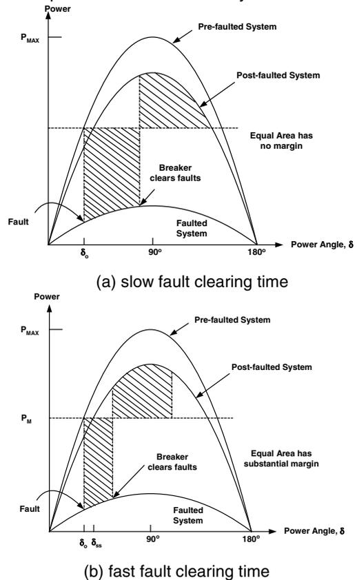
Fig. 7. Effect of Fault Clearing Time
