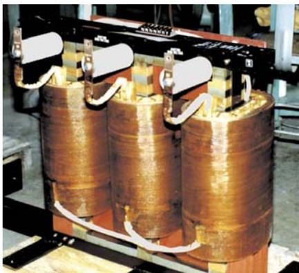
Figure 4. Excitation Power Potential Transformer
