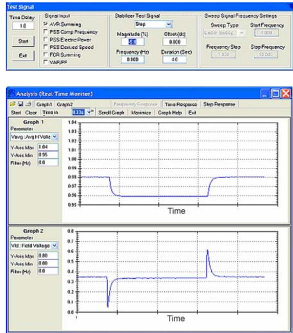
Fig. 10. 5% Voltage Step Change in Voltage Regulator Mode
