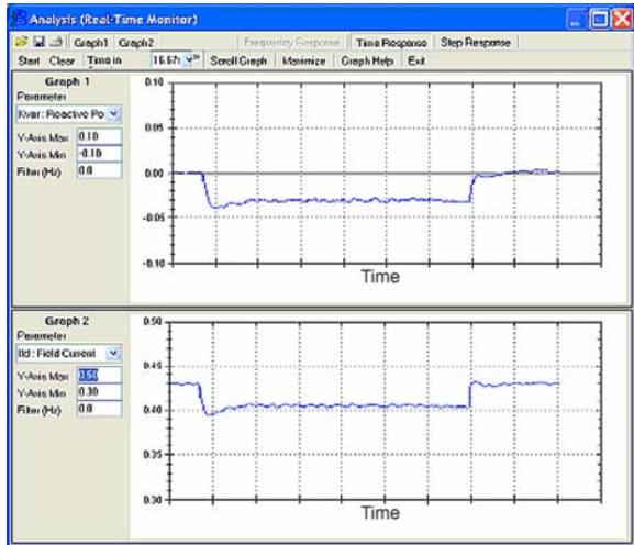
Fig. 11. Under Excitation Limit Dynamic Step Test
