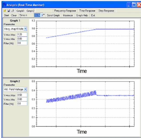
Fig. 9. Voltage Buildup in Voltage Regulator Mode
