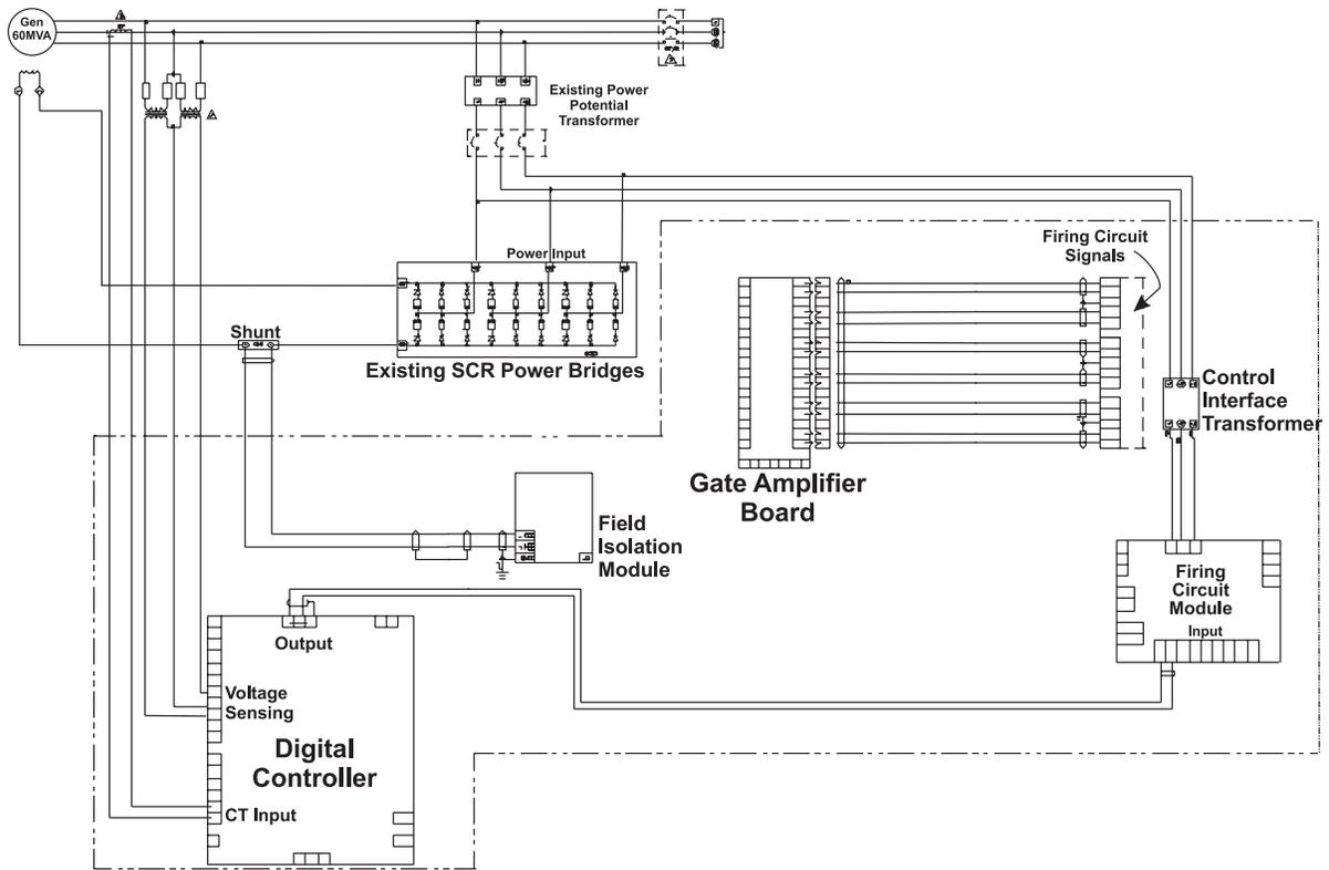
Fig. 7. Partial schematic of the new interconnected system
