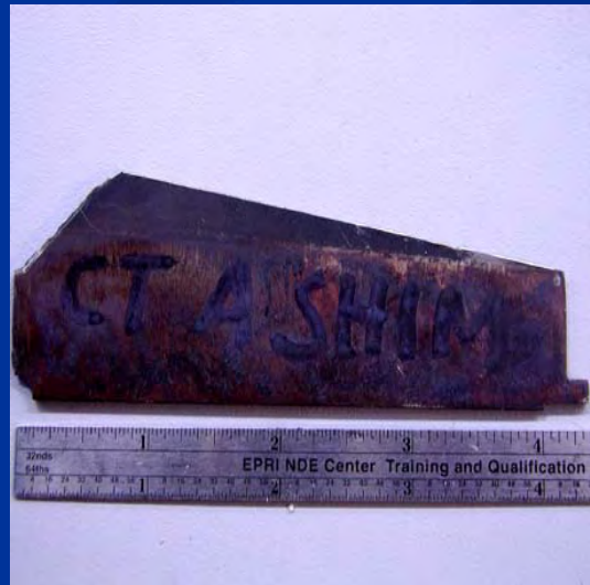
Photograph Of Shim After Removal
