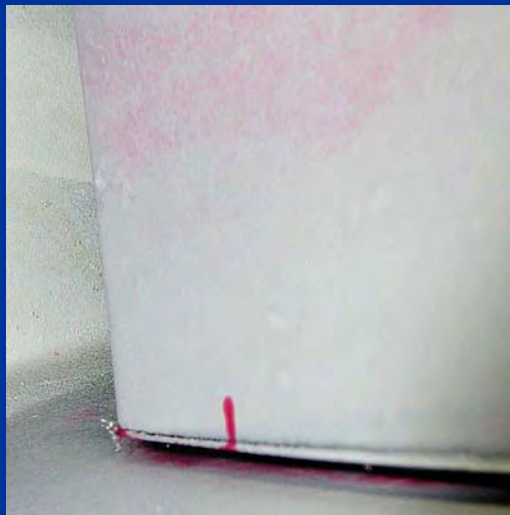
Radial Tip Crack Identified By A 1509-1 PT Examination
