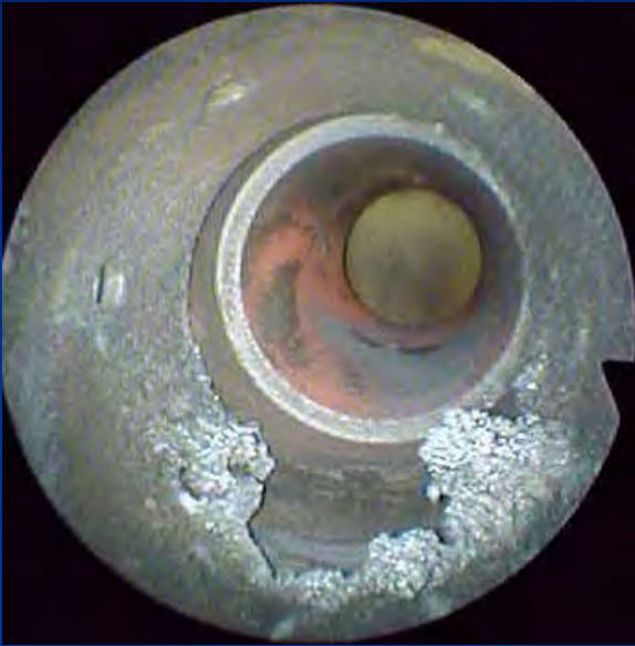
Melted Crossfire Tube
